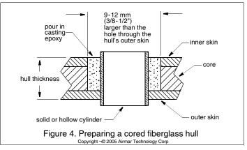
the outside. (If the hole is drilled in the wrong location, drill a second hole in a better location. Apply masking tape to the outside of the hull over the incorrect hole and fill it with epoxy.)
