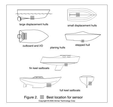
· Choose an accessible spot inside the vessel with adequate space for the height of the housing, tightening the nuts, and installing the insert. Allow a minimum of 280mm (11").
