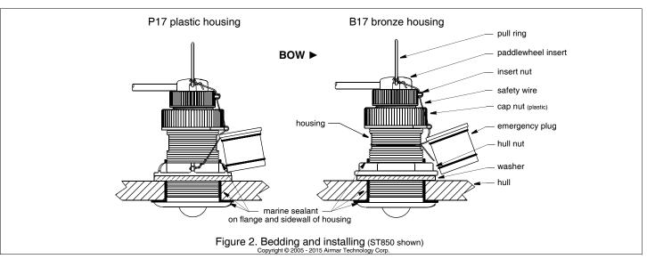
**ST850**—Be sure the notch on the upper rim of the housing and the corresponding arrow on the flange are still pointing forward toward the bow.
