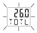
If no action is performed within twenty (20) seconds the unit will return to the normal operating mode.
