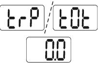
The trip log value may be reset without changing the total log value. if the total log is reset to zero, then the trip log will automatically reset to zero.
