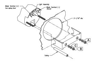
**NOTE:** To change the light bulb, twist out black socket assembly one-eighth turn counterclockwise until it pops out. Bulb pulls straight out of assembly. It is a GE No. 161 instrument lamp.
