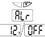
Press and hold both keys for three seconds and the displayed value will begin to flash.
